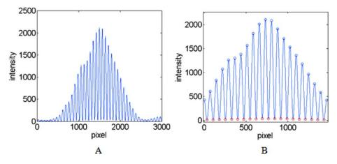
FIG. 1. (Color online) (A) Smoothed interference pattern. The slight asymmetry in the interference pattern was due to minor misalignments in the optical apparatus. (B) Center segment, with minima and maxima identified. The y-axis is the level of illumination intensity returned by the Thorlabs camera.
